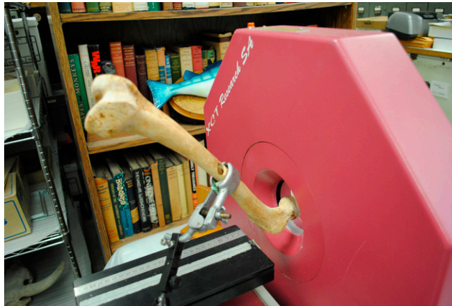
Fig. 54. Positioning of the femoral head in the pQCT scanner, shown as an example of the pQCT setup that ensured homologous scanning of the same position and plane in each specimen.
