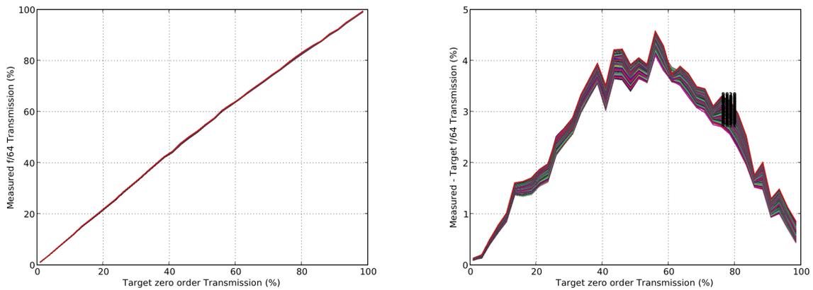
Figure 8. 10  $\mu\text{m}$  microdot patch transmission accuracy for all 40 OD patches: *Left*: target vs. measured *Right*: target vs. measured minus target.
