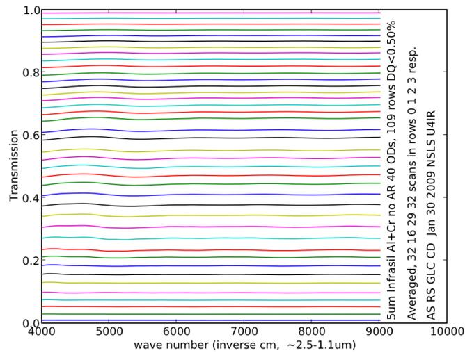
Figure 5. Spectra of uniform optical density (OD) calibration patches fabricated with 5  $\mu\text{m}$  metallic microdots.
