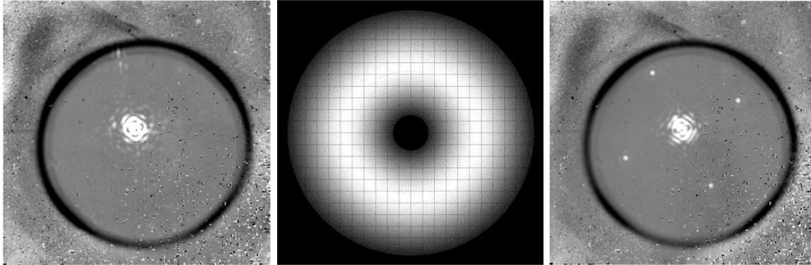
Figure 10. *Left:* A  $1.65 \mu\text{m}$  coronagraphic image used without an astrometric grid in the pupil. *Middle:* Microdot apodizer with an example of a fine opaque grid. *Right:* A  $1.65 \mu\text{m}$  coronagraphic image showing the coronagraphic PSF and the first set of four satellite spots generated by such a grid in the pupil.
