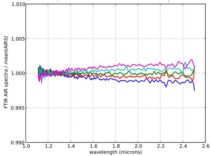
Figure 2. Five sequential spectra through air relative to the mean of all five spectra. Temporal variations like these must be calibrated out by taking reference spectra at appropriate intervals. Such calibration does not work well across fills of the electron ring, which occur about 4 to 5 times in 24 hours.
