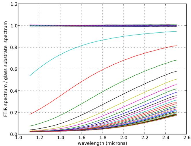
Figure 3. Spectra of a continuous opacity material on Infrasil substrate. The opacity can be a strong function of wavelength, possibly because the opacity is confined to a superficial layer on the glass.
