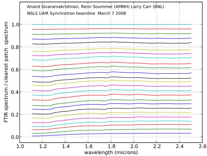
Figure 4. Spectra of uniform optical density (OD) calibration patches fabricated with 2  $\mu\text{m}$  metallic microdots. Chromaticity is far less than for the continuous opacity material, but is still visible from the fact that the curves are not horizontal.
