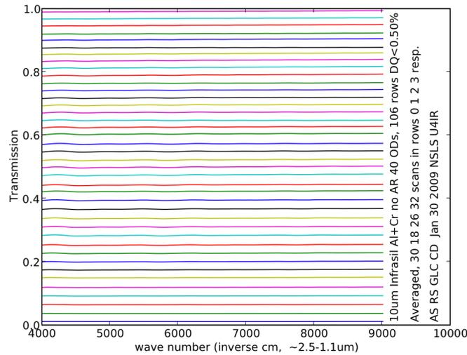
Figure 6. Spectra of uniform optical density (OD) calibration patches fabricated with 10  $\mu\text{m}$  metallic microdots.
