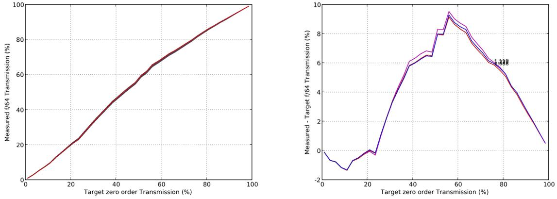
Figure 7. 5  $\mu\text{m}$  microdot patch transmission accuracy for all 40 OD patches: *Left*: target vs. measured *Right*: target vs. measured minus target.
