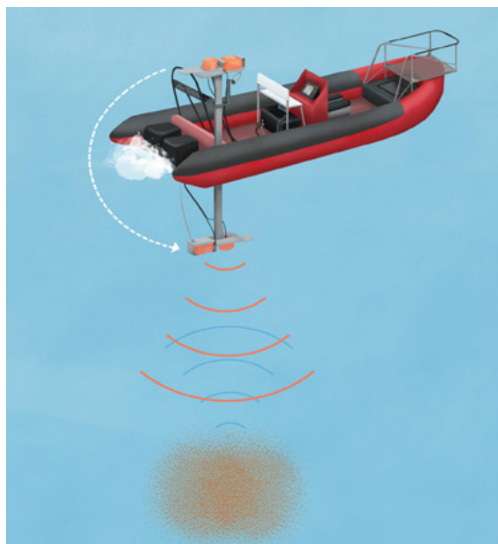
Figure 1. Echosounder. Once placed in the water, the instrument sends down pings of sound (orange curves) that bounce off whatever they encounter, then measures the amplitude of the echoes (blue curves) and the time it takes for them to return to the instrument. Higher-amplitude echoes mean there’s more material; longer waits mean it’s farther away.
