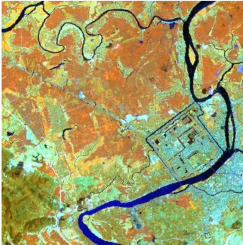
Figure 4.3: Landsat TM (WRS-2) Path = 125 Row = 49, April 21, 2003, The city of Hue in Vietnam. Red=4, Green=5, Blue=3
