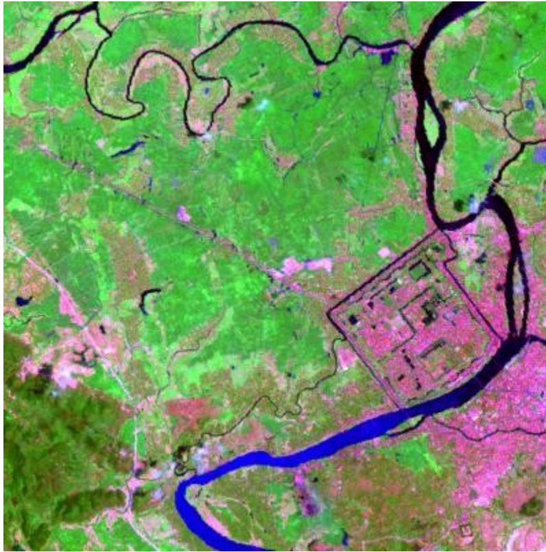
Figure 4.4: Landsat TM (WRS-2) Path = 125 Row = 49, April 21, 2003, The city of Hue in Vietnam. Red=7, Green=4, Blue=2
