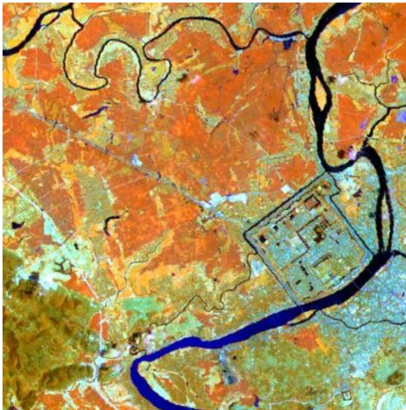
Figure 3: Landsat TM (WRS-2) Path = 125 Row = 49 April 21, 2003 Bands 4, 5, 3 represented with red, blue and green The city of Hue in Vietnam In this image the town of Hue, Vietnam is colored light blue. The reddish brown color in the lower left portion of the image is forest and the orange patches throughout the image represent grass, shrubs, and rice. The blue and black linear features are rivers, streams, and a moat around the old city of Hue.
