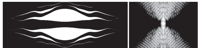
Fig. 13. (a) This optimized pupil mask has six openings within an elliptical envelope designed to match the pupil of TPF-C (section 6.9). (b) The corresponding image plane diffraction pattern, showing a strongly suppressed central star, and dark-hole areas (on the left and right) with residual intensities below a theoretical contrast of 10^{-10} . The IWA is 4\lambda/D and the throughput is 30%.
